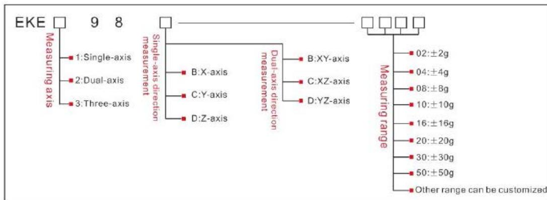
E.g.: EKE198B-02: single-axis、X Axis direction measurement、 $\pm 2g$  selection
